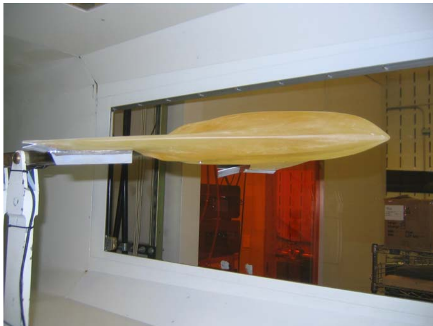
Figure 54: Lambda Model with +20^\circ Symmetric Flap Deflections, AOA = 0^\circ
