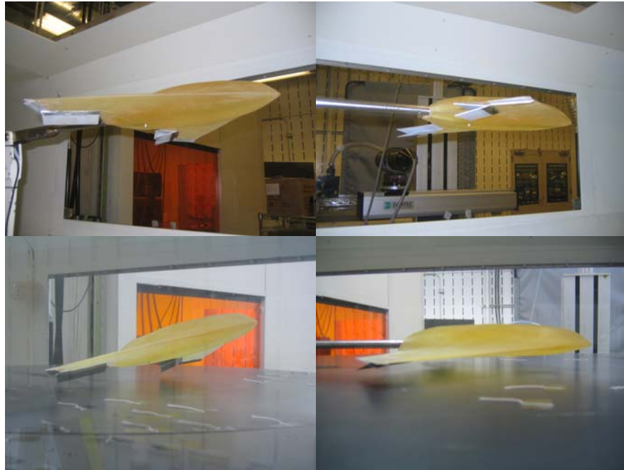
Figure 7: Four Views of the \frac{1}{2} - Scaled Lambda Model OGE and IGE ( h/b = 0.05 ) with Mid/Outboard Trailing Edge Split Flap Deflections
